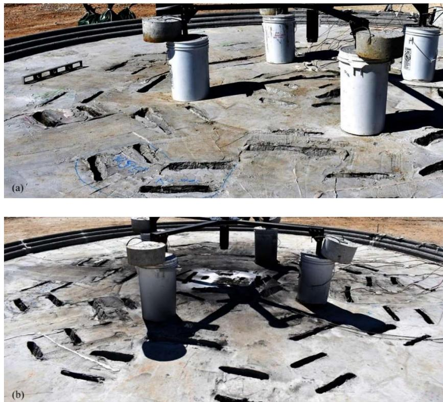
*Figure 1a – 1b: Photos taken of the Lunar PAD before (a) and after (b) the hot-fire test. Enhanced contrast for clarity.*
