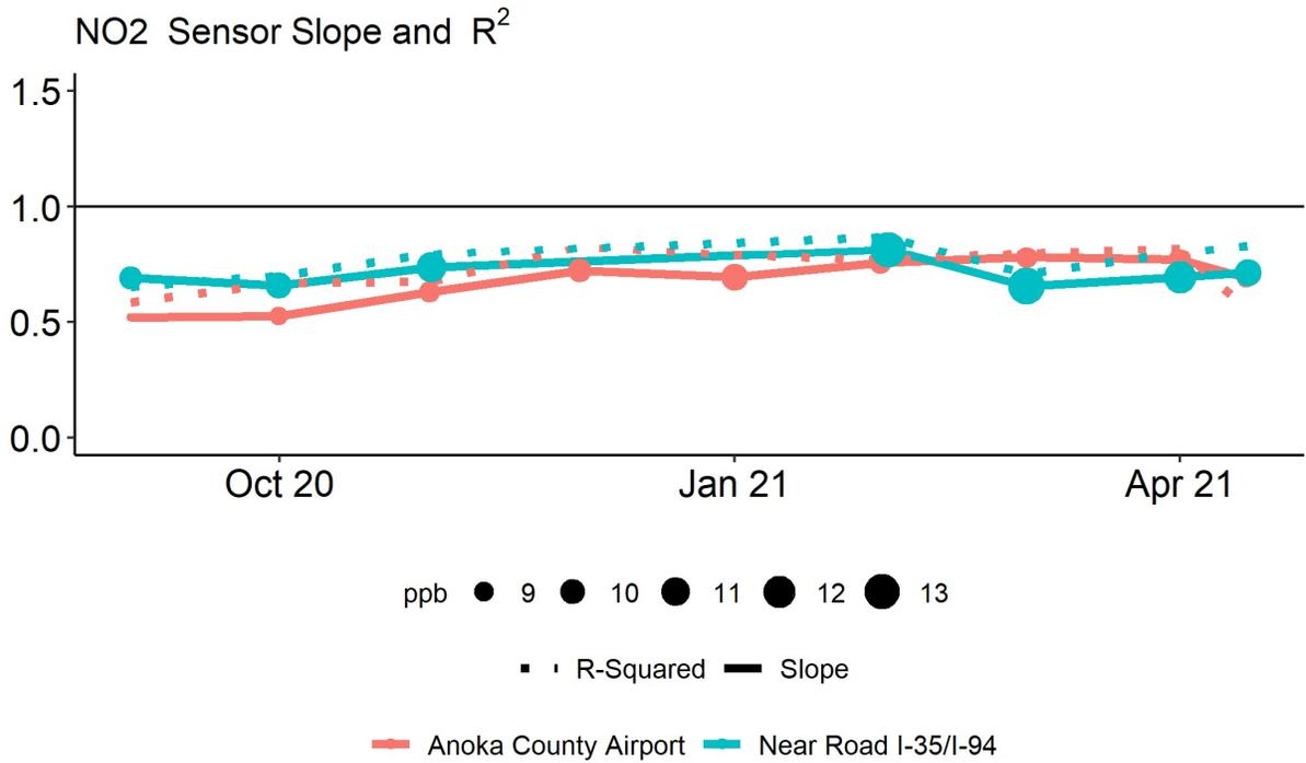
Figure 8 NO2 sensor slope, R<sup>2</sup>, and average concentration over time at the 35W site and the Anoka Site using RF correction.
