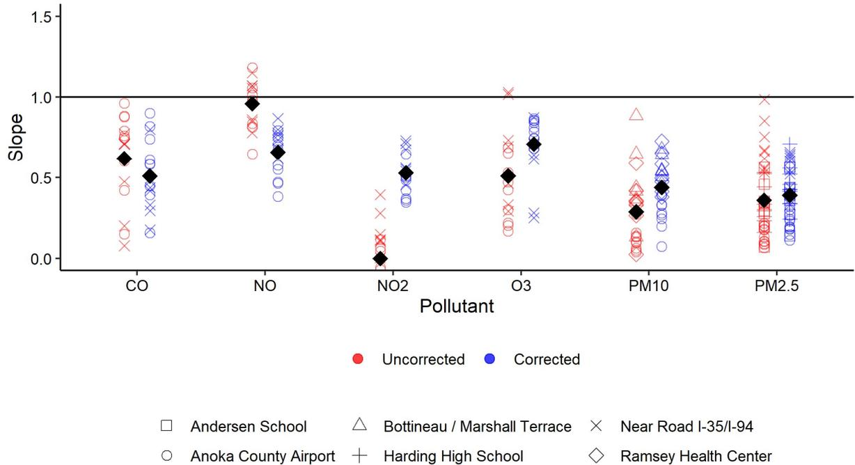
Figure 10 Slope of line between federal reference sensor and AQ Mesh sensor before and after Neural Network Correction applied. Each point is one month at a specific site and the black squares are the mean of the measurements.
