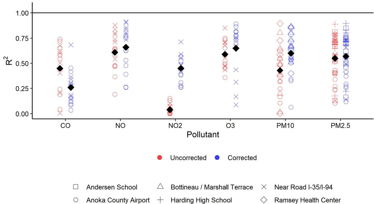
Figure 11 R-Squared of Neural Network correction for sensors compared to a federal equivalent. Black dots represent the mean of the measurements in the column.
