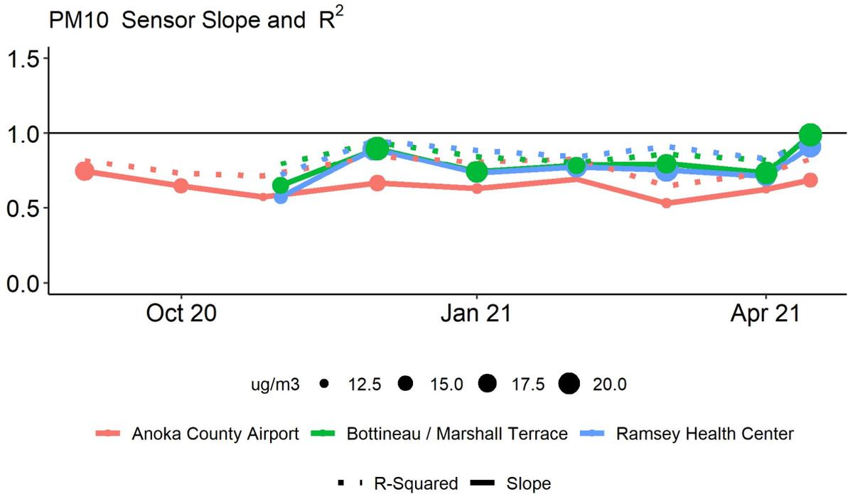
Figure 9 PM10 sensor slope, R<sup>2</sup>, and average concentration over time at the Ramsey Health Center (RHC) site, the Bottineau Marshall Terrace site, and the Anoka Site using RF correction.
