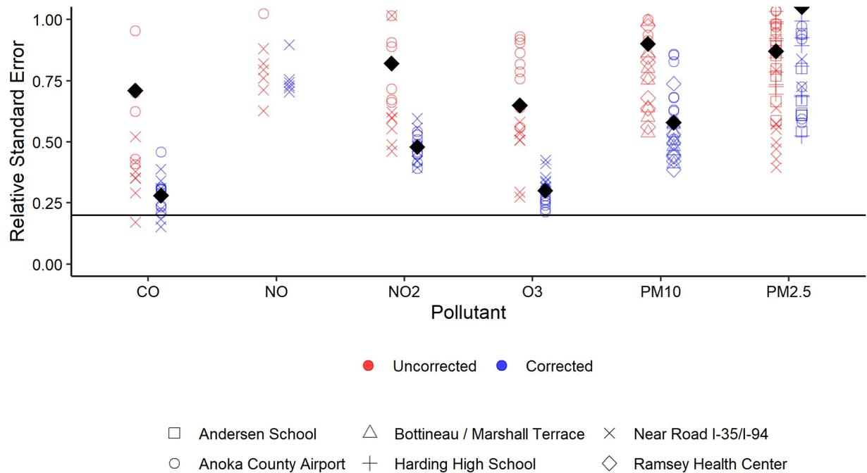
Figure 12 Relative Standard Error of sensors after a Neural Network correction is applied, with black markers for the average. The target to reach is zero, but an RSE of under 0.2 is a goal for many low-cost sensors.
