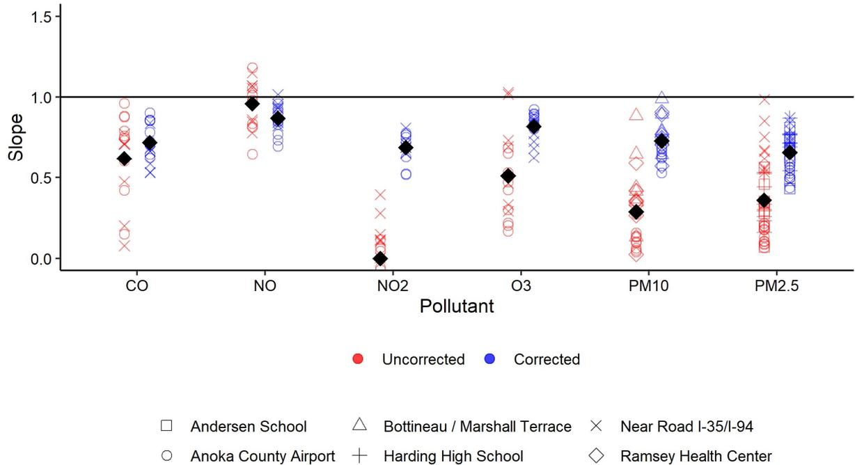
Figure 5 Slope of the line between federal reference sensor and AQMesh sensor before and after Random Forest Correction applied. Each point is one month at a specific site, and the black squares are the mean of the measurements.
