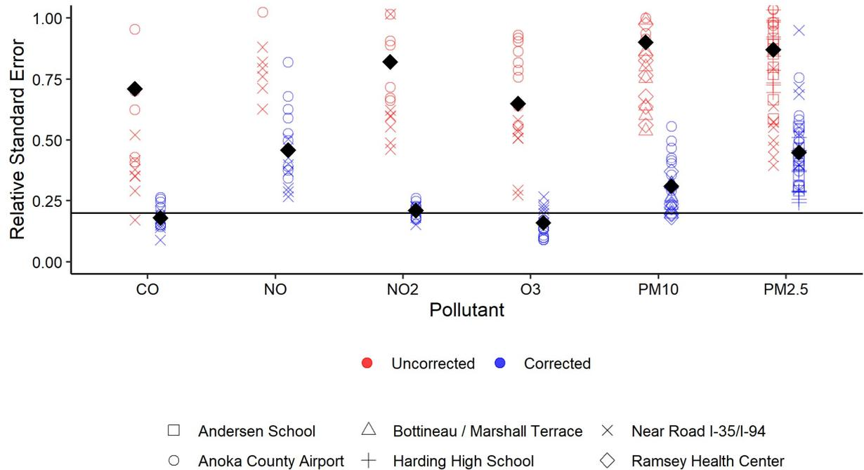
Figure 7 Relative Standard Error of sensors after a Random Forest correction is applied, with black markers for the average. The target to reach is zero, but an RSE of under 0.2 is a goal for many low-cost sensors.
