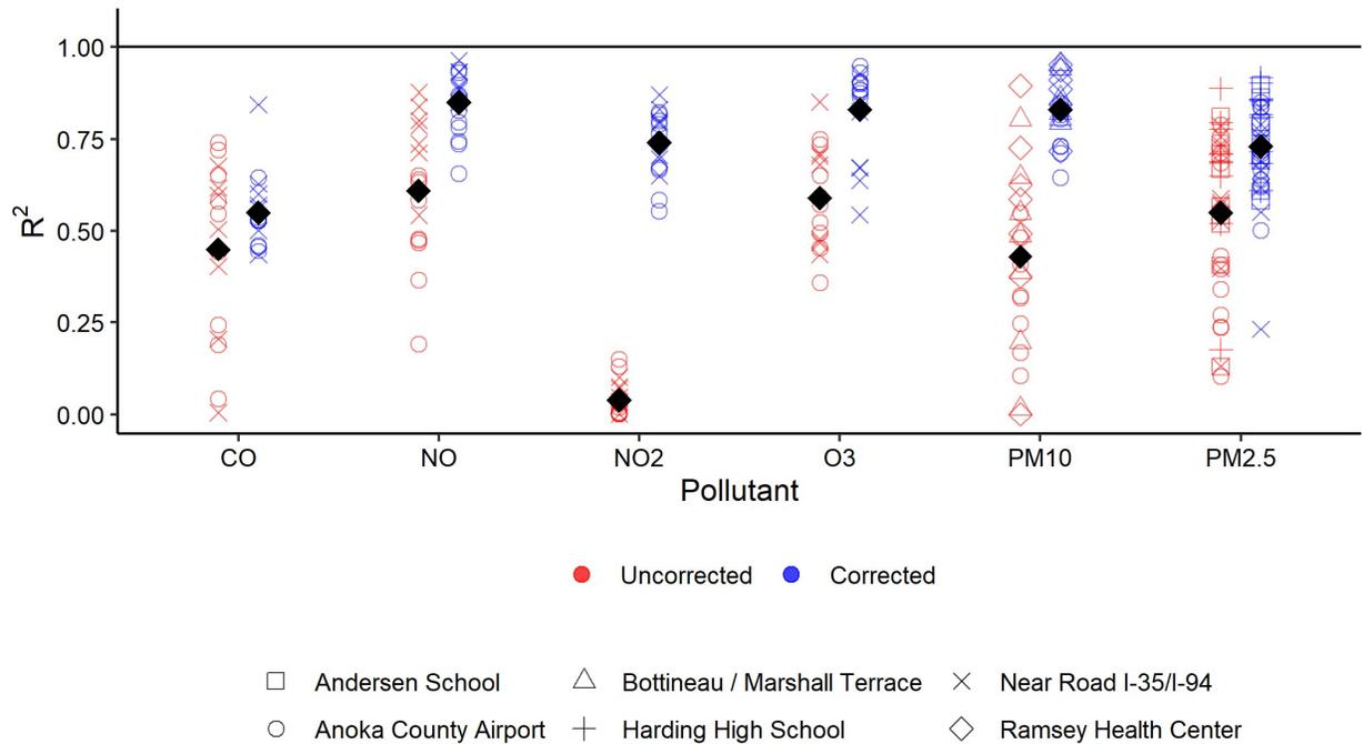
Figure 6 R-Squared of Random Forest correction for sensors compared to a federal equivalent. Black dots represent the mean of the measurements in the column.
