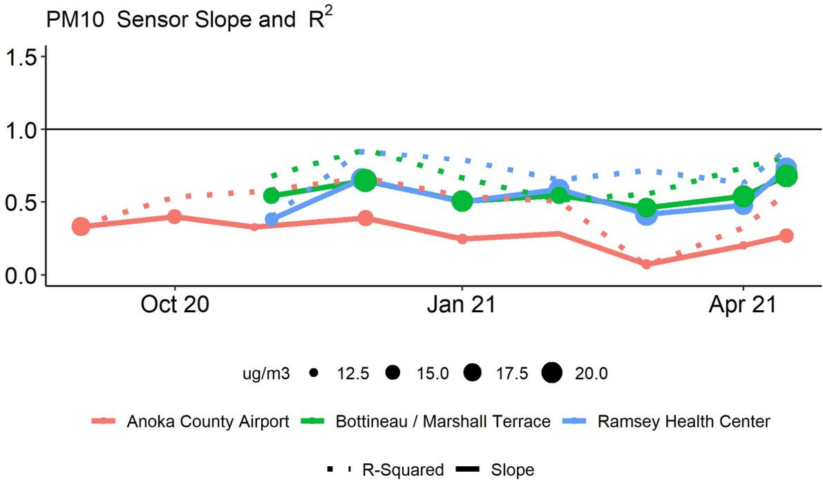
Figure 14 PM10 sensor slope, R<sup>2</sup>, and average concentration over time at the Ramsey Health Center (RHC) site, the Bottineau Marshall Terrace site, and the Anoka Site using NN correction.
