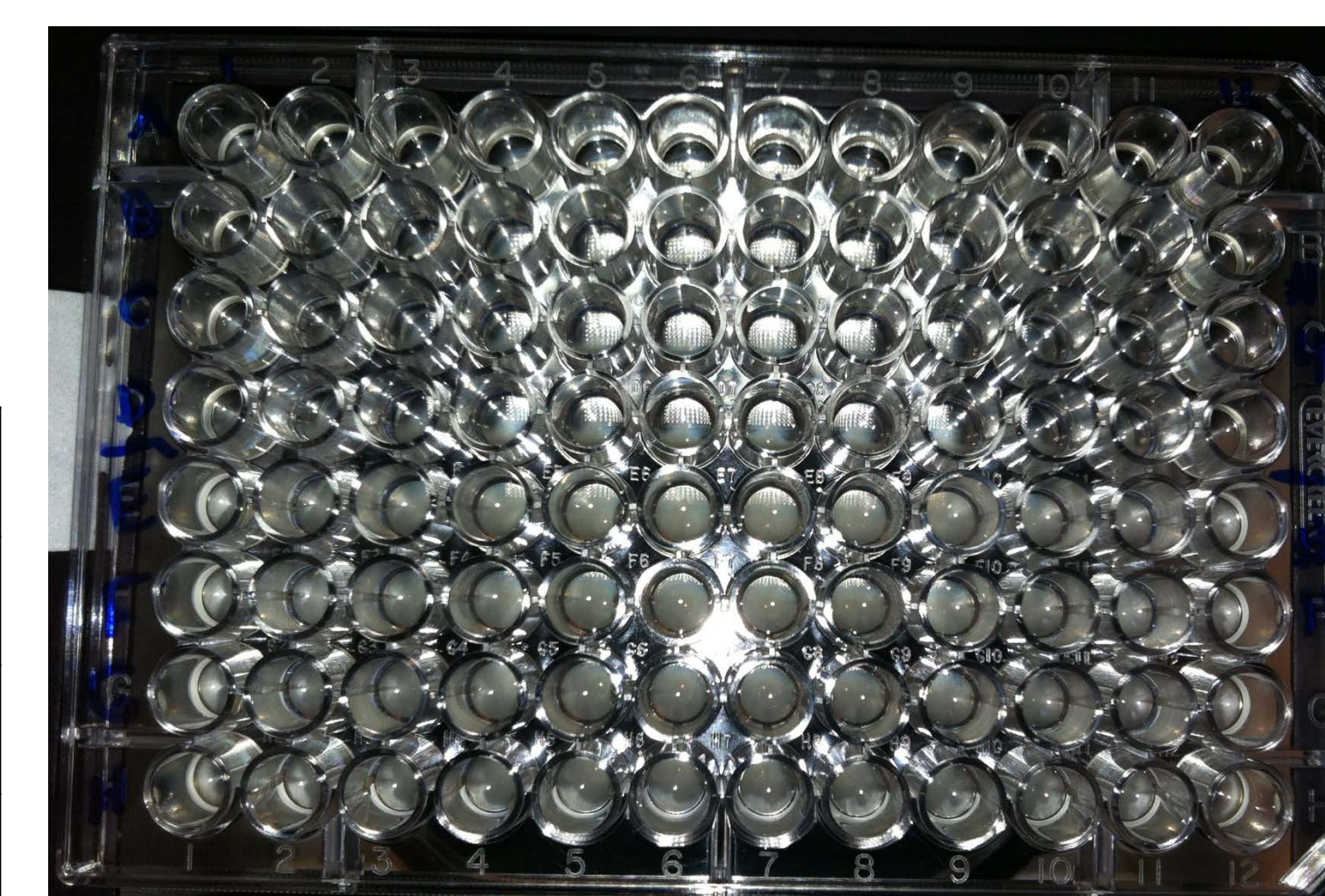
Figure 3. MIC testing. Two-fold serial dilutions ranging from 32 to 0.016 µg/ml (left to right) were prepared. The isolates in the top 4 rows had an MIC of < 0.016 µg/ml, and the MIC of the isolate in the bottom 4 rows was > 32 µg/ml.
