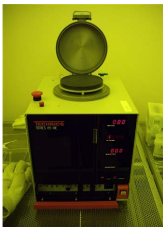
Fig. 5. RIE system in Microelectronics Fabrication Laboratory, Minnesota State University Mankato.
