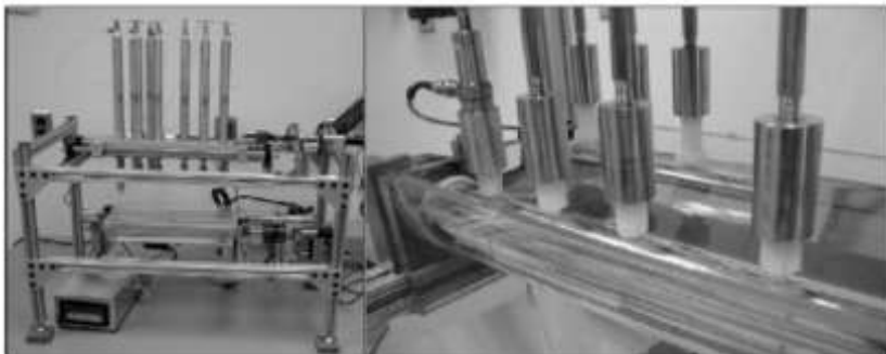
Figure 8: DAWS machine (left) and close-up of sample holders and shaft (right) [3]
