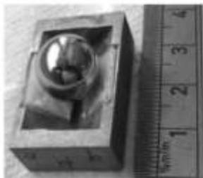
Figure 13: Prism loaded with two specimens and counterpart ball [7]
