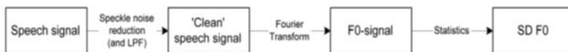
Figure 3. Processing Scheme for Emotional Prosody Measurement (EPM). This is the filtering method From Van Den Broek's (2004) study which extracted base frequency values of emotive speaking voice (p. 119). Also, see Table 1 .
