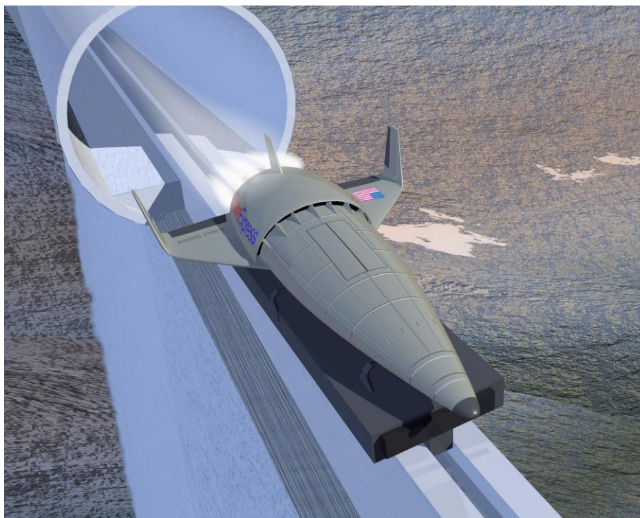
Figure 8. An artist's concept of a fictional RBCC-equipped SSTO utilizing MAGLEV catapult-rail system. Image courtesy of NASA/Marshall Space Flight center (NASA-MSFC).
