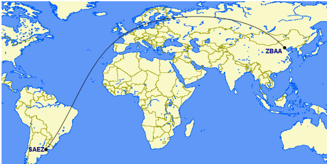
Figure 3. Great circle (geodesic) route SAEZ to ZBAA (EZE to PEK) on conformal cylindrical Mercator chart. Courtesy of GC Mapper. Maps generated by the Great Circle Mapper ( www.gcmap.com ) - copyright © Karl L. Swartz.
