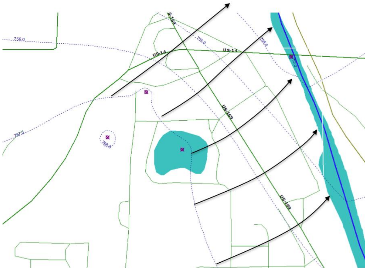
Figure 14. GFLOW model results showing estimated subsurface water flow for Hiniker Pond and surrounding areas, North Mankato, MN
