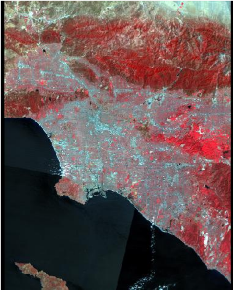
Figure 3.4: The Los Angeles Metropolitan area 1989 image as downloaded through USGS and converted into image format through ERDAS. There is clear cloud coverage along the Pacific coastline, which was classified separately to distinguish its spectral reflectance from the other classifications.
