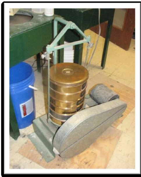
Figure 4.05: The Gilson Ro-Tap Sieve Shaker prepared for an analysis with a stack of Tyler brass sieves.
