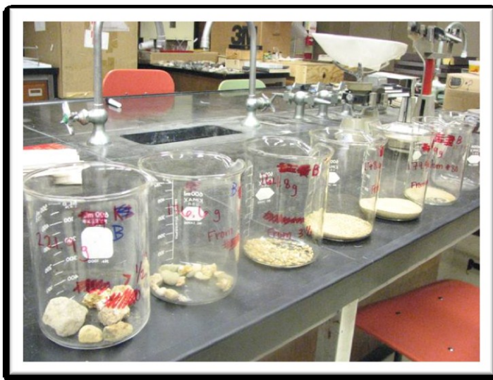
Figure 4.06: Sieve size fractions split into separate beakers.
