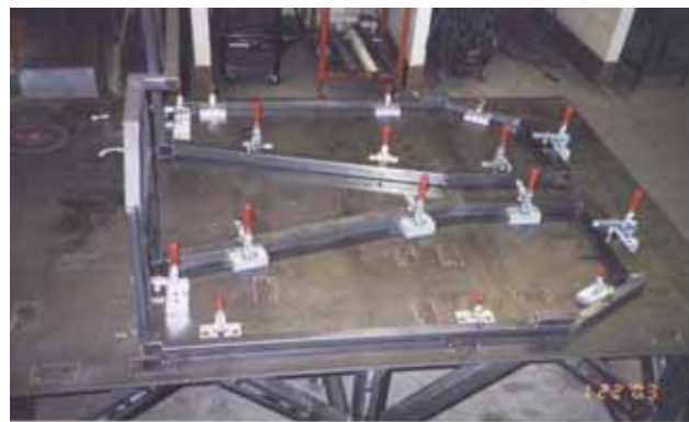
Figure 4, Chassis jig table, fixtures and clamps.
