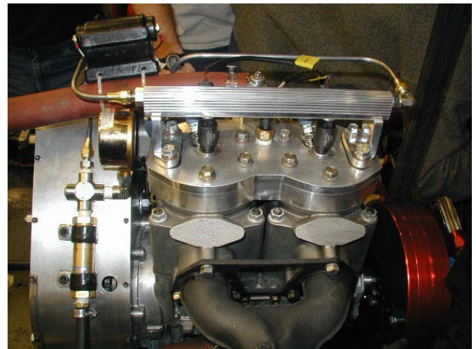
Figure 9: DFI Engine with Fuel Pump Drive on Left
