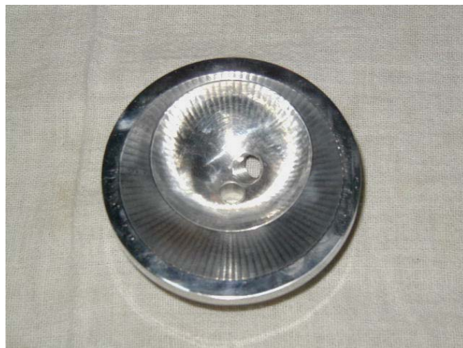
Figure 6: Squish Area and Combustion Dome Orientation
