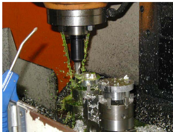
Figure 5: Machining of the Combustion Chamber
