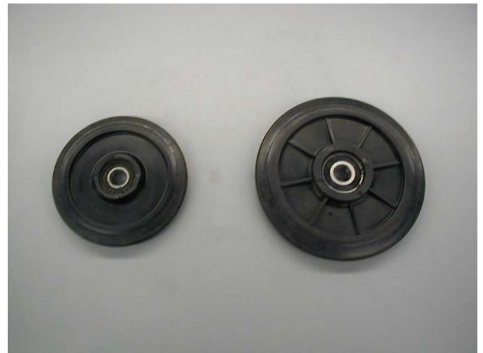
Figure 13: Original Idler Wheel (left) New Idler Wheel (right)
