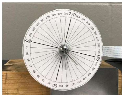
Figure 14. The angle indicator shown on the right view side of the testing apparatus. The three positions used to measure the electrical signal response were 210^\circ , 220^\circ and 240^\circ degrees.
