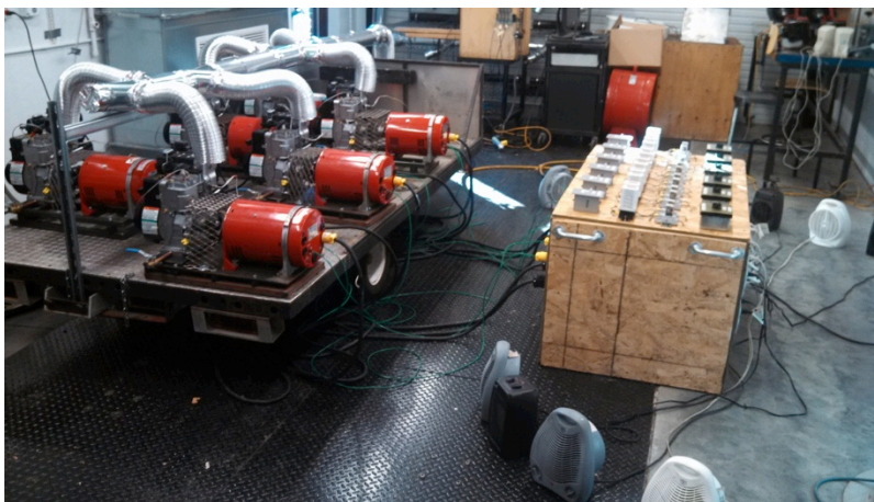
Picture 2 shows the engines on the aging apparatus and the load being switched by the circuitry.
