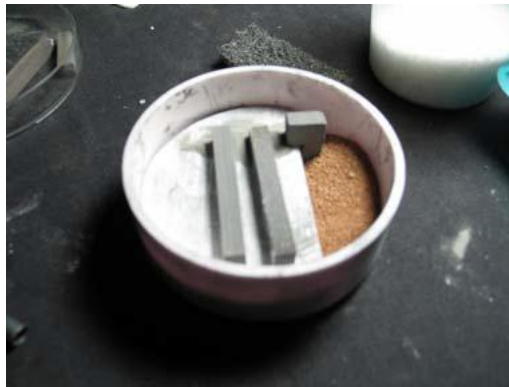
Figure 8 Sintered Part and Powdered Bronze (ExOne, 2013)
