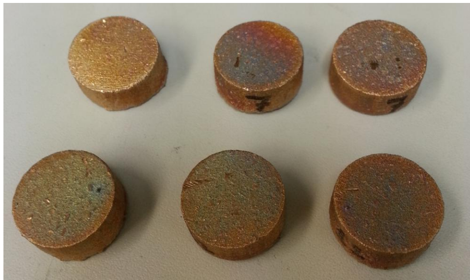
Figure 20 Disks Prior to Finish Machining
