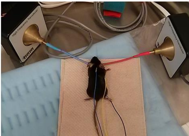
Figure 3. Standard ABR setup with electrodes subdermally attached to the mouse. The blue electrode is positioned at the vertex of the skull, the yellow is positioned at the mastoid below the ear, and the black electrode is positioned along the thigh. Sound is channeled into the ears of the mouse with high-frequency transducers.
