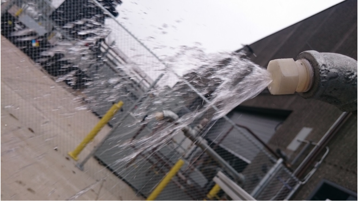
Figure 67 Water droplet formation at the nozzle
