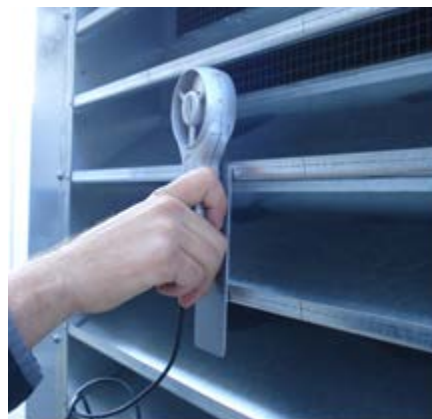
Figure 39 Anemometer is attached to a flat plate, so that the air flow is parallel to the anemometer.
