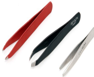
Picture 9: Tweezers (third class levers)
