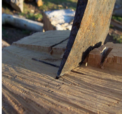
Picture 5 Axe (example of a wedge)
