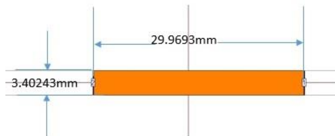
Fig. 12 Geometry of Microstrip Transmission Line
