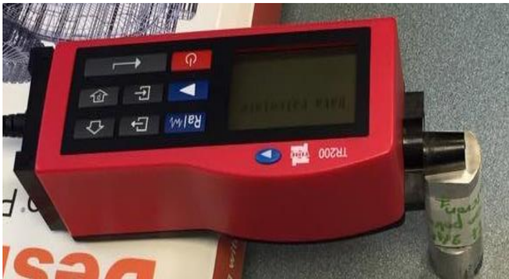
Figure 2.2-5: Portable surface roughness tester TR200 used for surface roughness measurement of aluminum surface.
