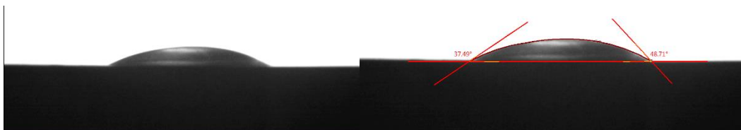
Figure 2.2-12: Illustration of contact angle formed on Aluminum surface (Used Grit Paper: 320, Surface Roughness: 0.59\mu\text{m} , Liquid: Castrol Oil).
