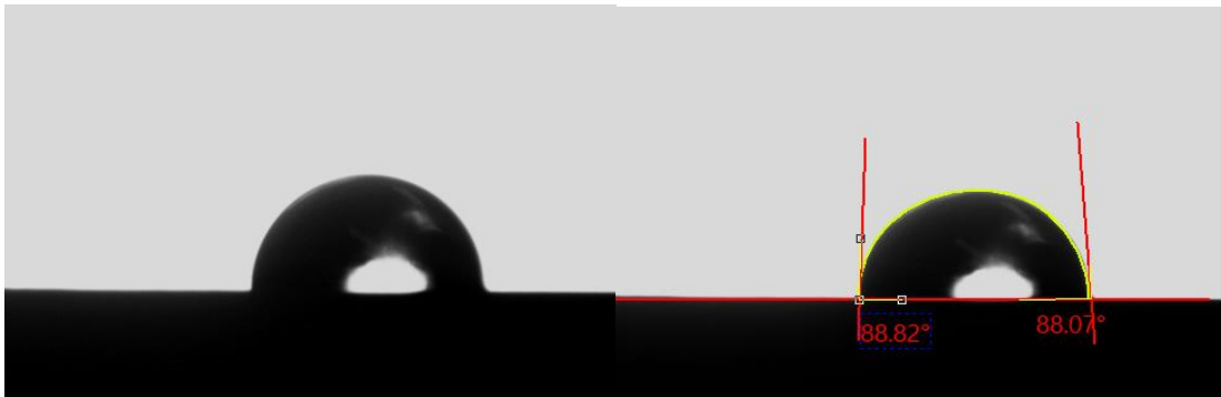
Figure 2.2-11: Illustration of contact angle formed on Aluminum surface (Used Grit Paper: 600, Surface Roughness: 0.22\mu\text{m} , Liquid: Water).
