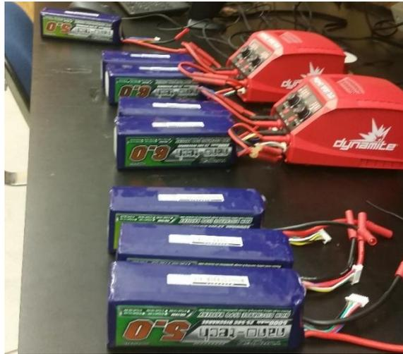
*Figure 5.13: Chain of Nano-Tech LiPo Batteries being charged*
