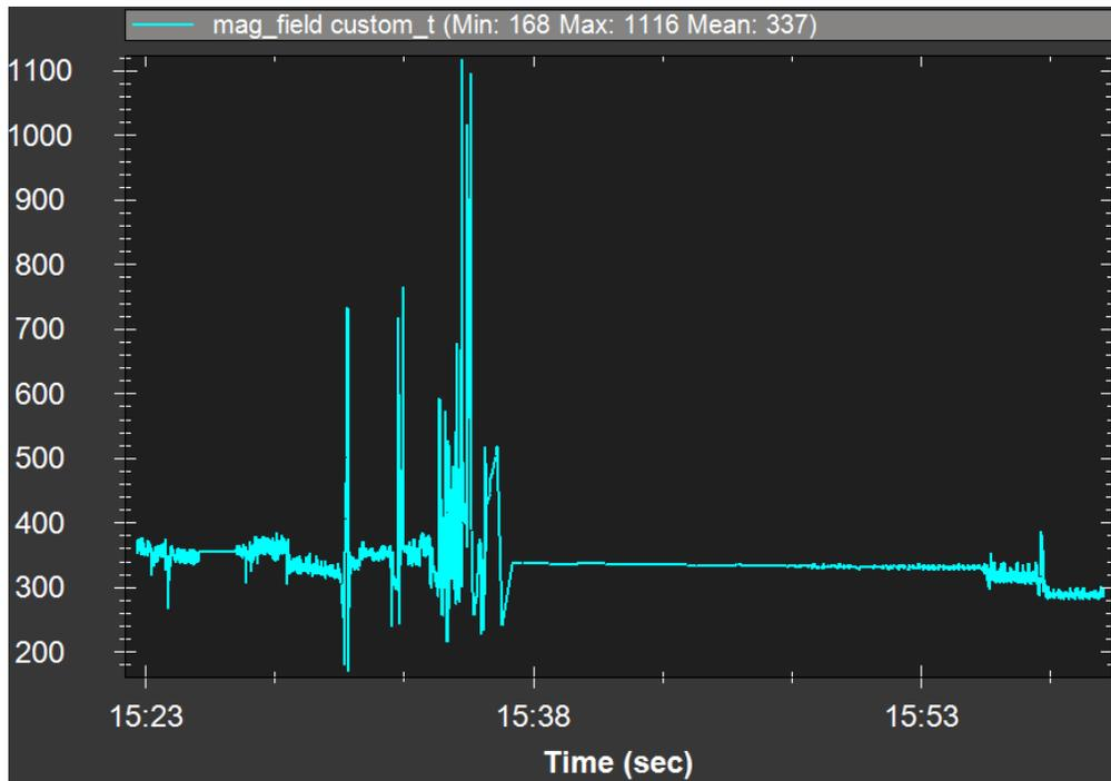
Figure 6.15: V2 Magnet interference (uT) during flyaway
