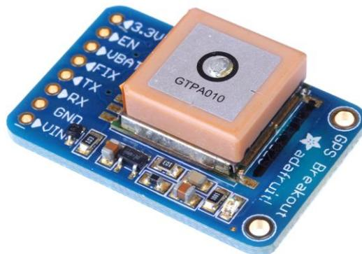
Figure 5.18: Adafruit Inc. GPS Breakout Board
