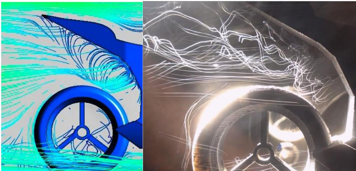
*Figure 23. Validation of CFD Results: Vortices Formation under Tail Section and Streamlines behind the Wheel.*
