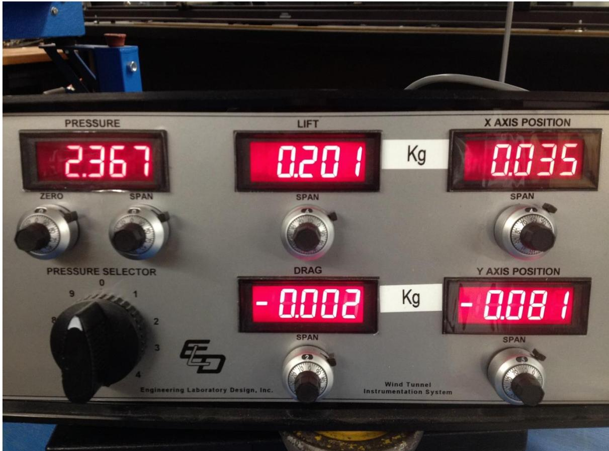
*Figure 29. Non-Wing Prototype Gauge Indication at Zero Wind Speed.*
