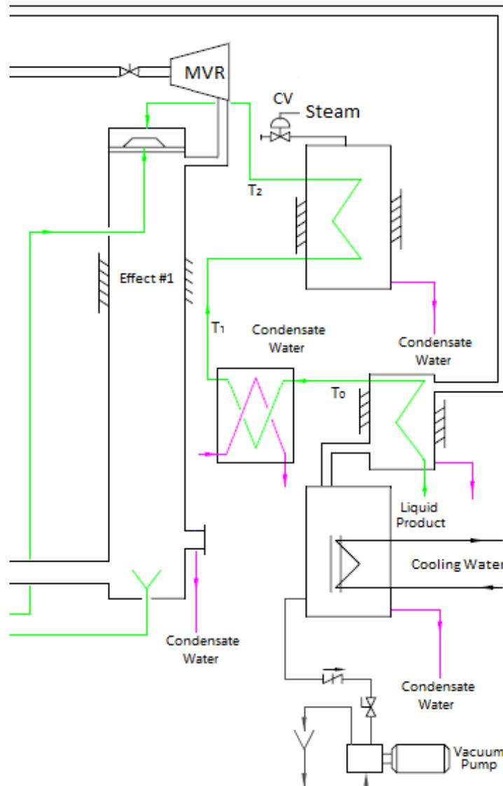
Figure 4. The data analyzed during the production batch is: 1.  $T_0$ , the discharge temperature of liquid product after the pre-heating step in new helical heat exchanger. 2. CV, the steam injection valve open percentage during the run. 3. Cooling water flow rate being sent into the condenser.
