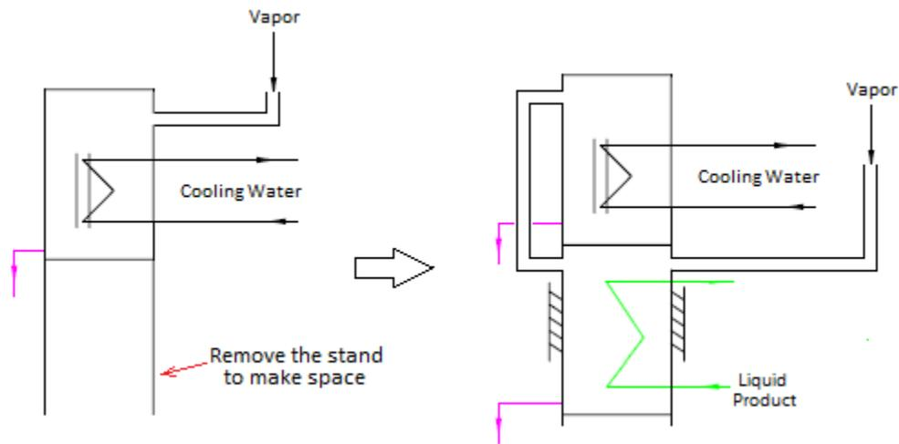
Figure 3. The schematic of the new heat exchanger installation.
