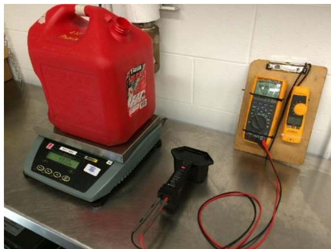
Figure 1 -Fuel being test using fuel composition meter
