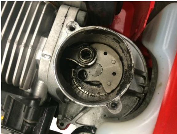
Figure 15-Removal of the crankcase cover
