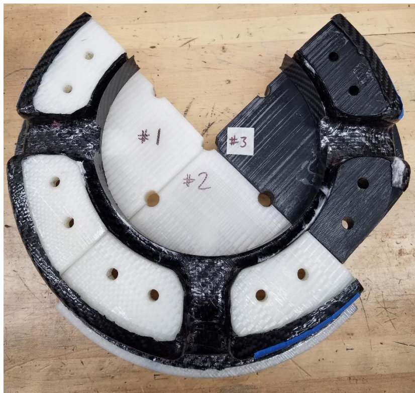
Layout of the mold materials, #1 & #2 are nylon and #3 is ABS
