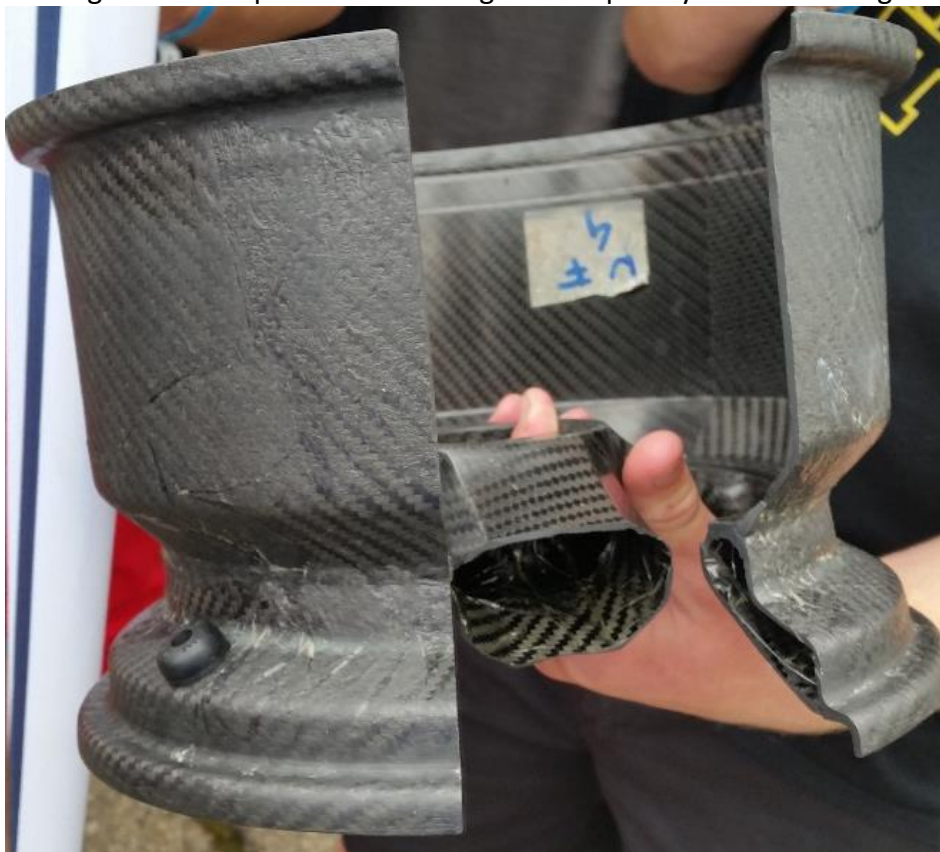
Figure 5 - Tu Graz Racing's hollow wheel section
