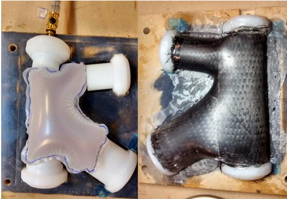
Figure 16 - Sculpted Cycles' use of an air bladder system (left) and a cured head tube (right).
