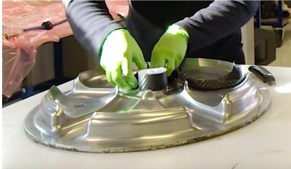
Figure 18 - An example of an aluminum mold from Koenigsegg
