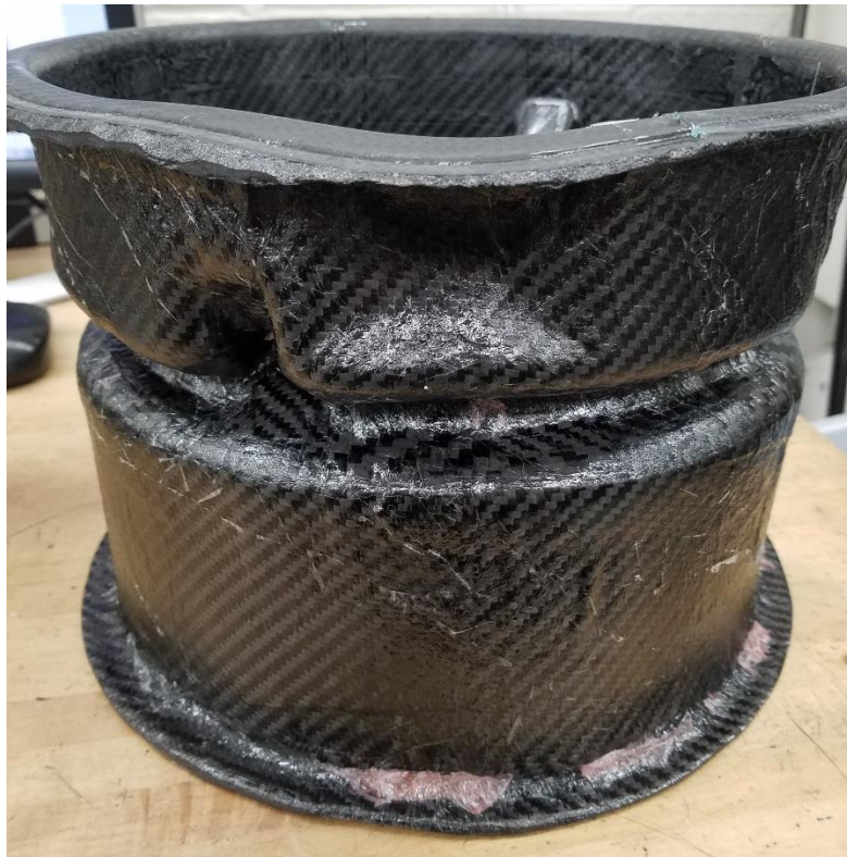
Distorted section of the laminate
