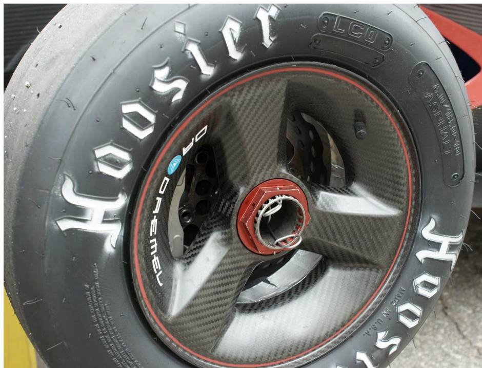
Figure 4 - Composite wheel design developed by Tu Graz Racing
