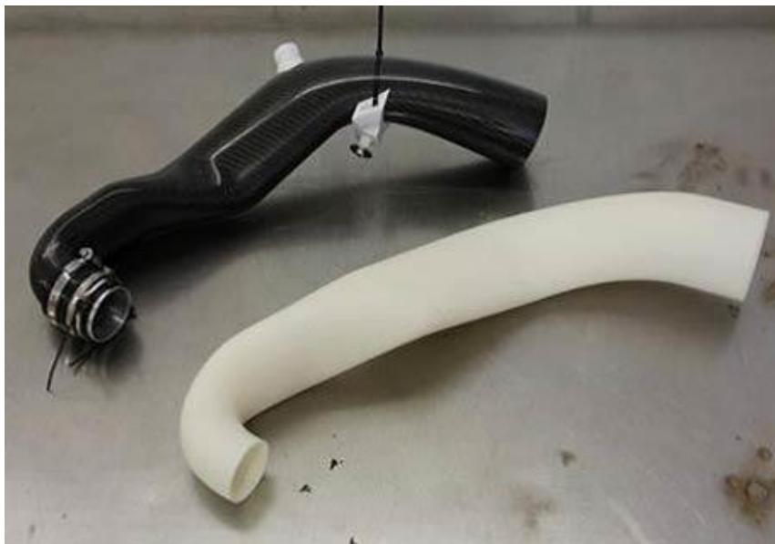
Figure 17 - Champion Motorsport's example of a printed soluble core
