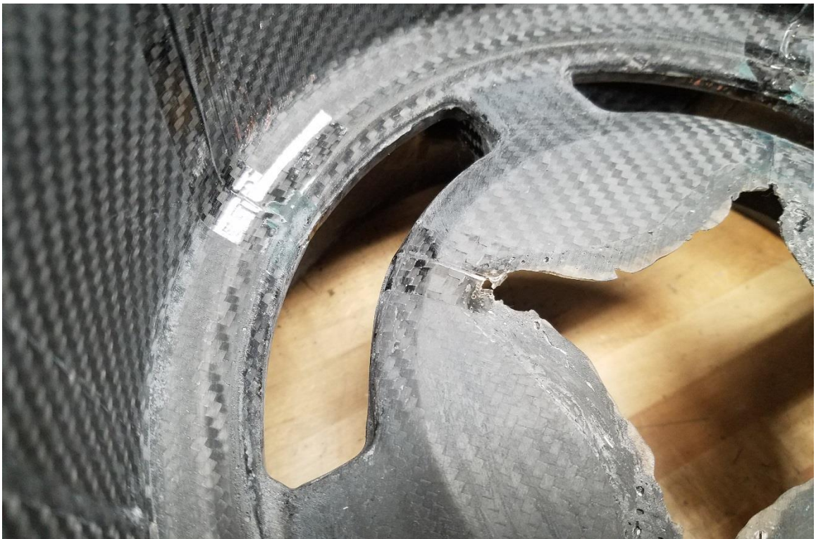
View of the inner half, laminate in the spoke area and around the center section have no apparent flaws.
