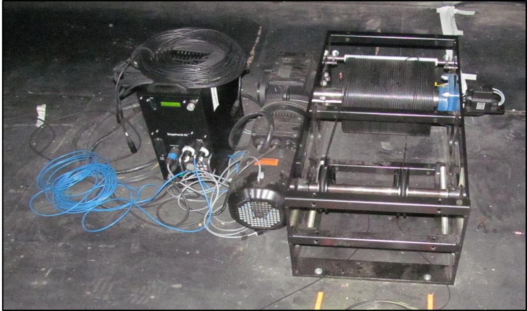
“PUSH STICK” DECK WINCH AND DRIVE BOX
