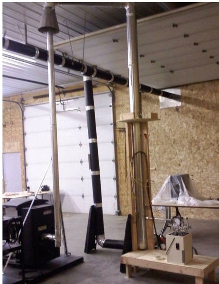
Image 19: Showing early stages of entire Method-28 and 5G dilution tunnel and test setup.
