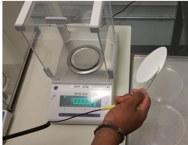
Image 18: Showing the analytical scale with covering to reduce draft and moisture affecting weight of PM sample filter.
