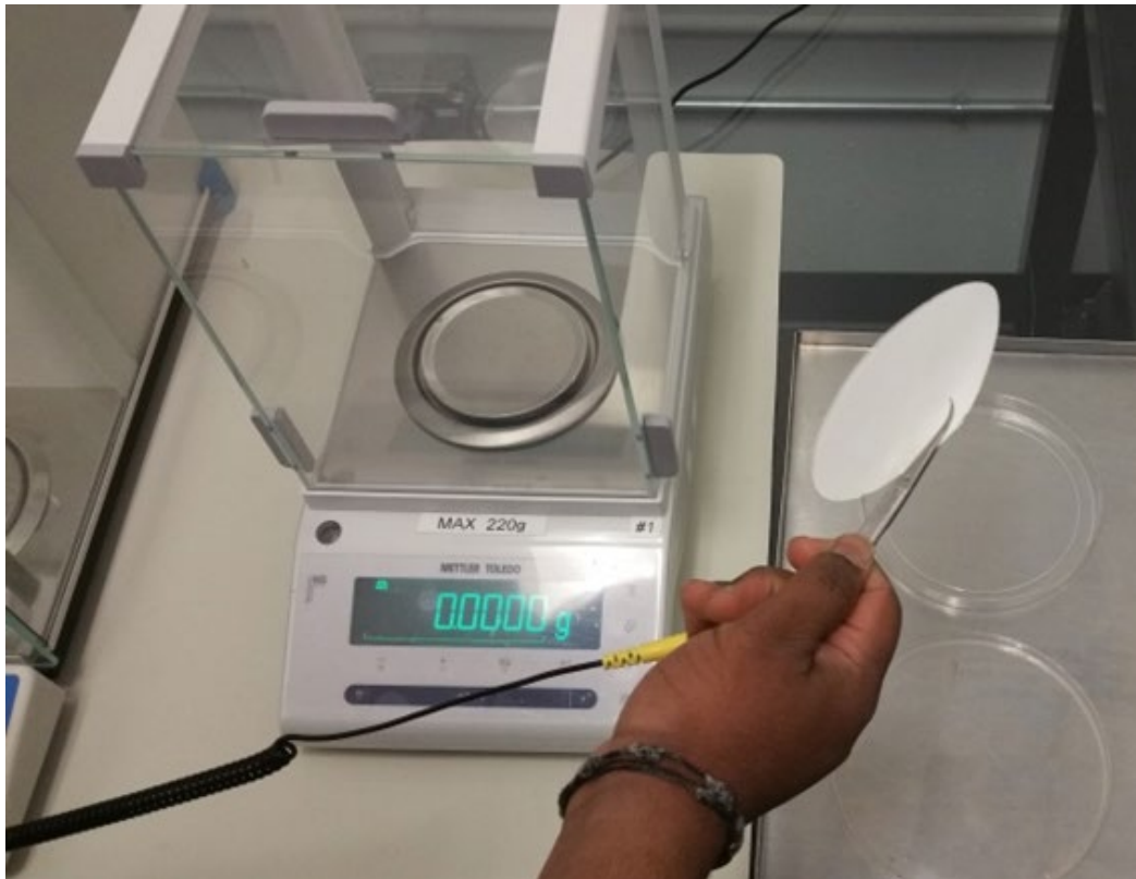
Image 10: Showing the analytical scale with covering to reduce draft and moisture affecting weight of PM sample filter.
