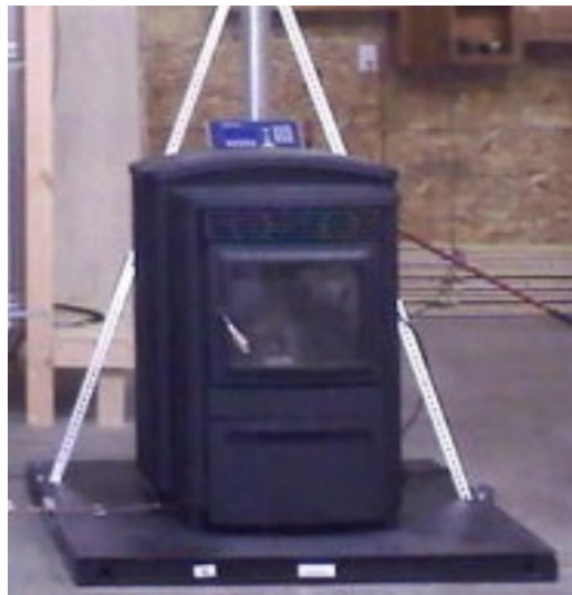
Image 9: The 310lb stove was shown here resting upon the scale. The stove boasted a 130lb hopper storage for pellet fuel.
