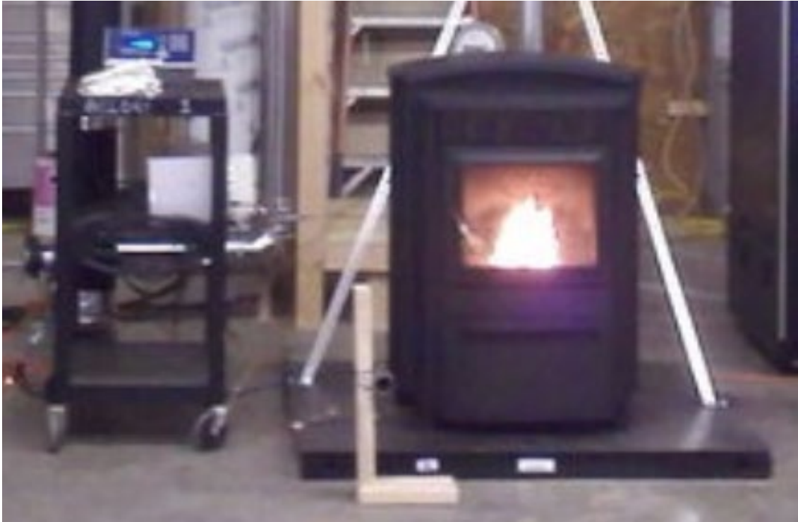
Image 14: The Hestia HHP2 resting on top of the Mettler-Toledo IND-560 platform scale.
