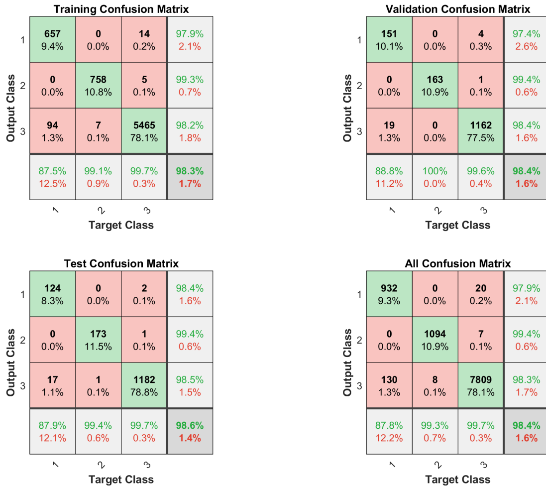
Figure 4-16: Confusion Matrix typical of Fault type 4 over 10000 training epochs
