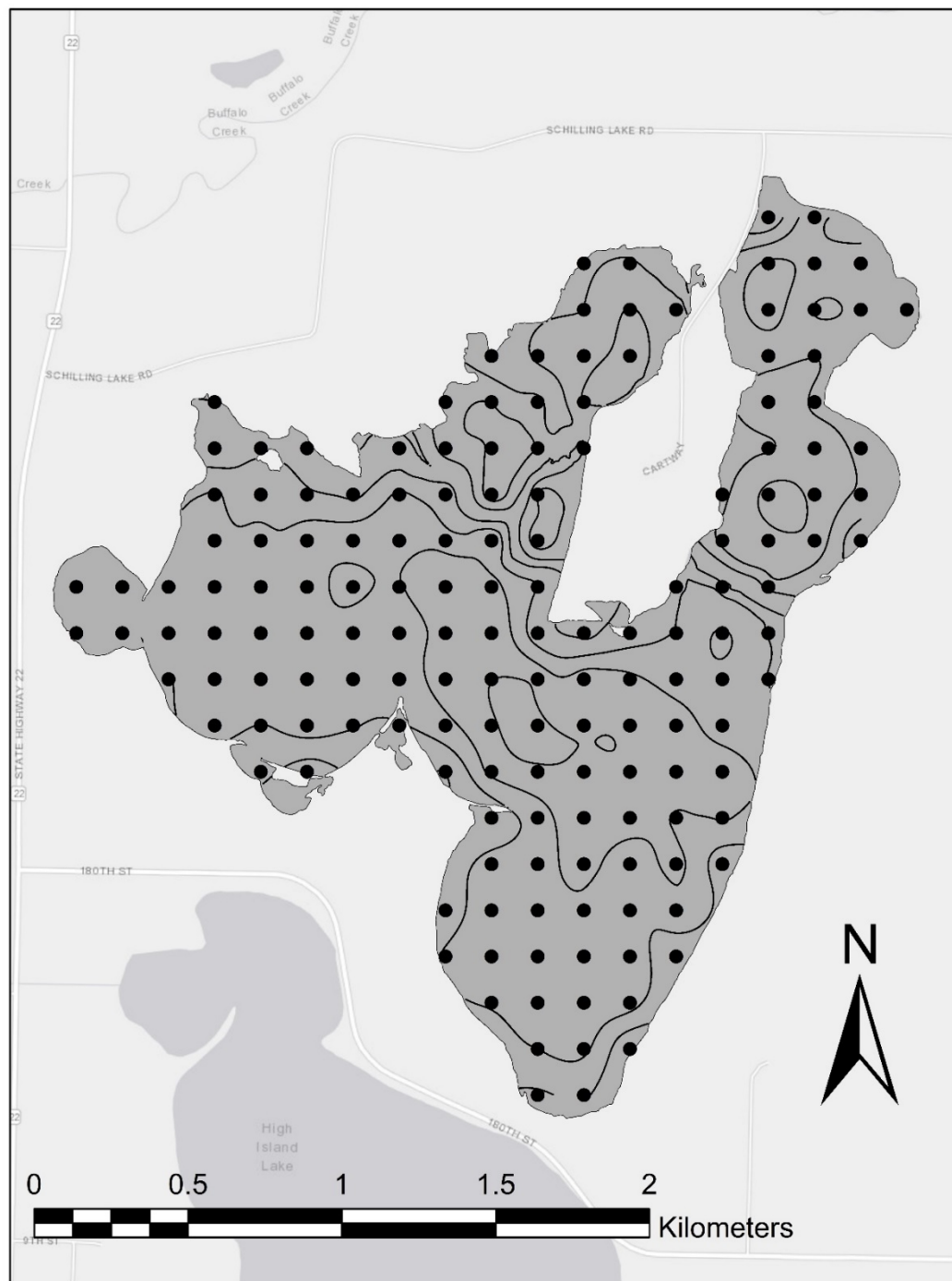
Fig 3.4 The grid of survey points in Schilling Lake for the surveys during the 2019 growing season in Sibley County, Minnesota. Contour lines represent changes of depth by 0.5m intervals. Contour lines derived from depth data at sample points (n=160).
