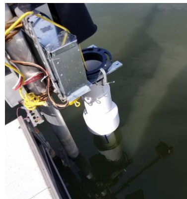
Figure 4.3: Image of the Hach DS5X multiparameter sonde in Bass Lake.
