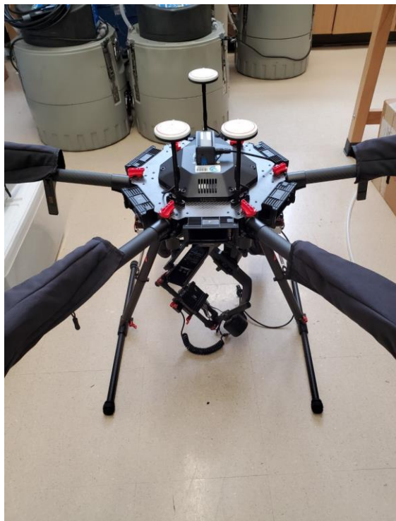
Figure 4.6: DJI Matrice 600 Pro UAV with DJI Ronin-MX gimbal mounted underneath.
