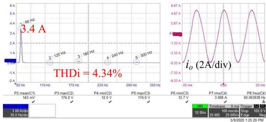
Figure 4.13 Spectrum of i_o when p_{in} = 420 W.
