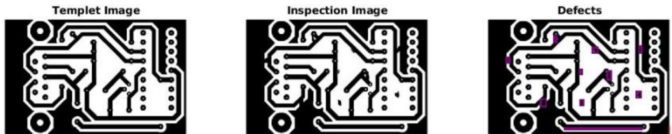
Figure 20 (Results from the defect detection of the Shorts, Excessive Shorts, Spurious Copper & Spur sample image)
