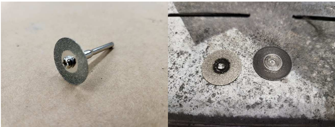
Figure 6. New cutting disc on the left. Worn out cutting disc on the right.
