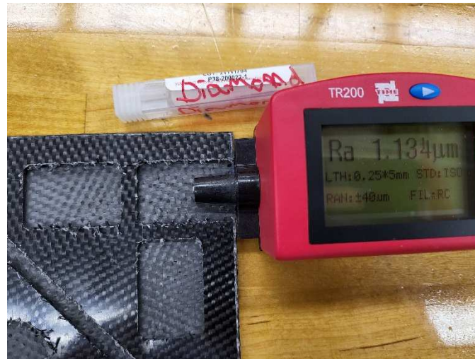
Figure 11. Using profilometer example. Checking the surface roughness of wet layup that was machined with the diamond endmill.
