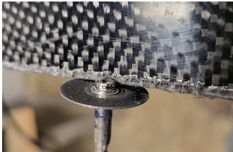
Figure 8. Example of the ruined edges due to the Dremel bolt.
