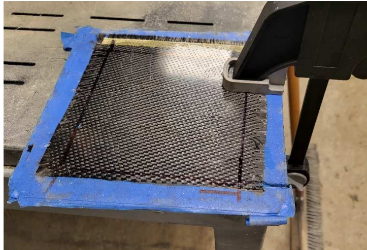
Figure 7. Carbon fiber test piece ready to be trimmed on ventilated table.
