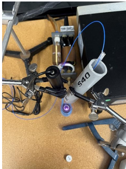
Figure 29: Combined MHT and PHT heating configuration, with laser turned on.
