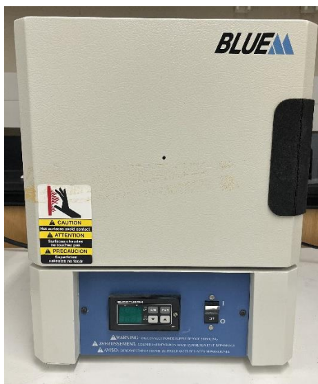
Figure 28: Oven used for hydrothermal silver decoration, Blue model BF51848A.
