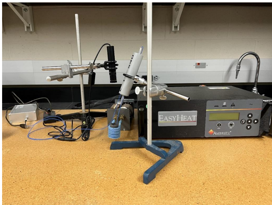
Figure 25: Configuration for both PHT and combined heating measurements. The alternating magnetic field is turned off while the laser, pictured above the coil, shines upon the ferrofluid.
