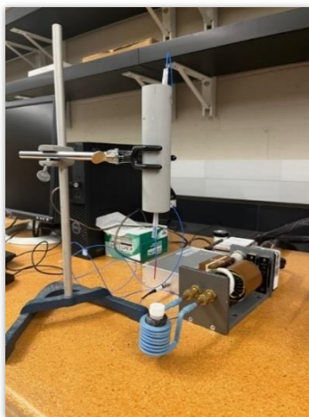
Figure 22: MHT set up, with optical fiber thermometer, tube, and current carrying coil.
