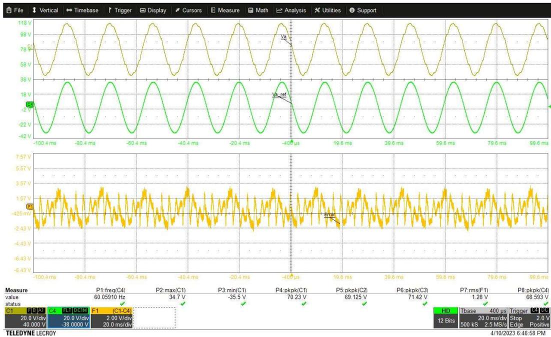
Figure 4.23: ANN-MPC reference tracking error with a nonlinear load.
