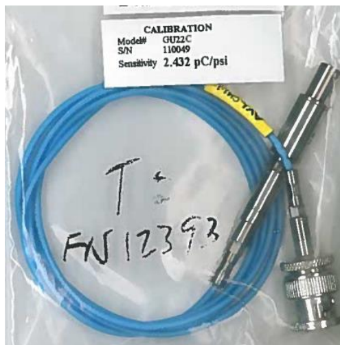
Figure 10 and 11: A calibrated pressure transducer before installation (10) and the AVL encoder installed on a test engine (11)
