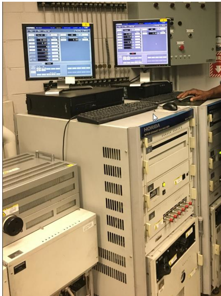
Figure 8: Horiba MEXA emissions measurement bench
