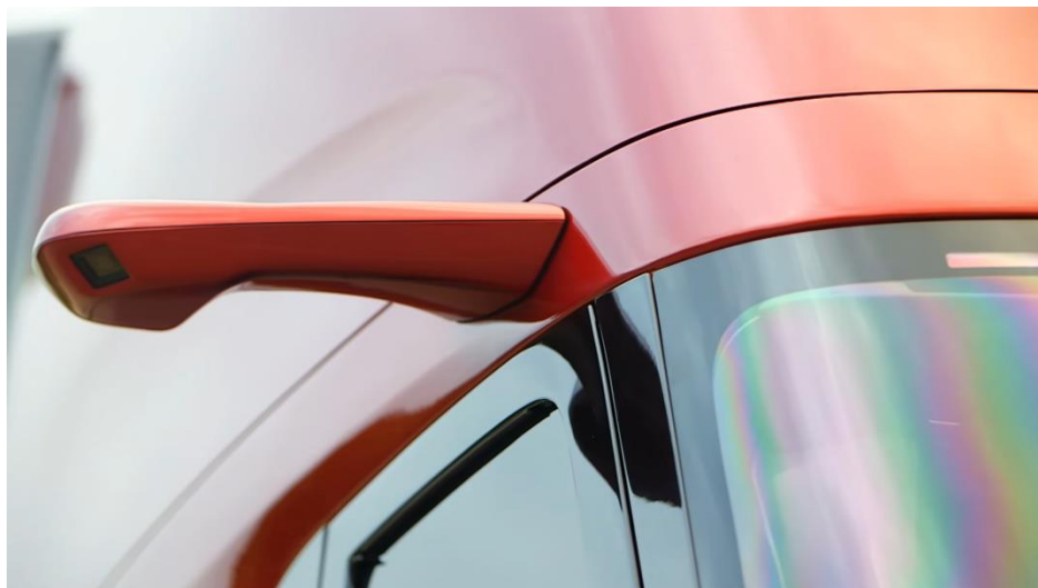
Figure 4: Rear View Camera
