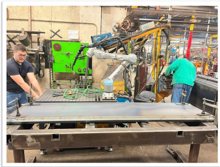
Tipper Tailgate Robotic Setup
