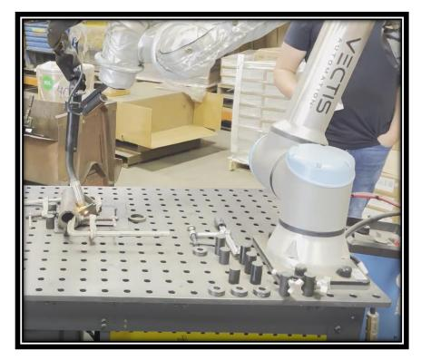
Should any discrepancies arise during the mock run, the mapping and coding process is redone to revalidate, ensuring the precise execution of welding tasks. Only upon successful revalidation does the welding process start.
